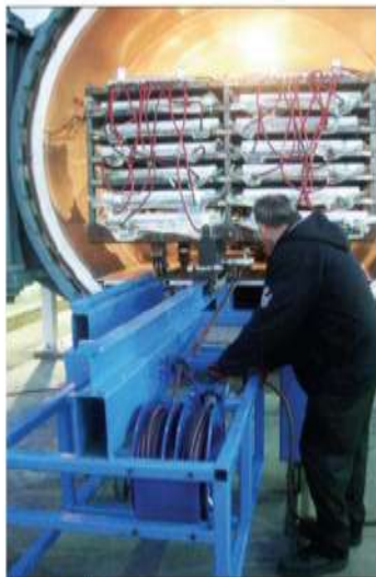
Workers manually move 8,000-pound racks into place. The new system (below) eliminates the need for employees to push the heavy racks.
