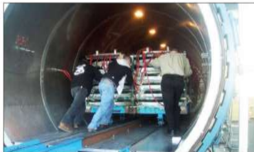
Workers manually move 8,000-pound racks into place. The new system (below) eliminates the need for employees to push the heavy racks.
